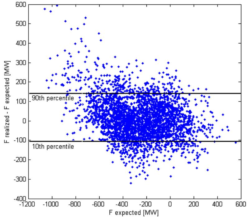
The distribution of the difference between the realized and the predicted flow ( $F_{\text{realized}} - F_{\text{predicted}}$ ) is shown in the graph below.
