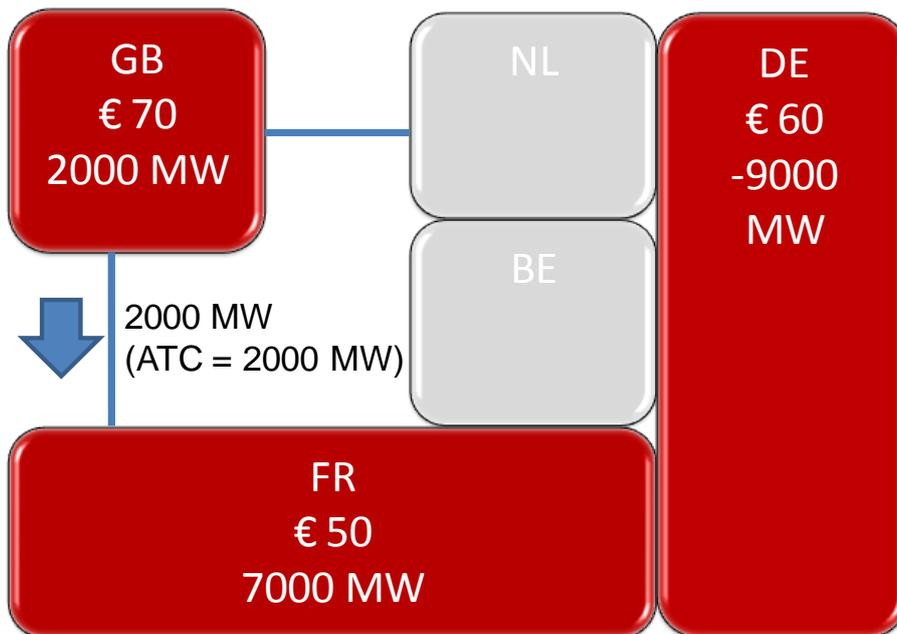
Figure 42: Example of advanced hybrid clearing with non intuitive flow on a DC cable.
