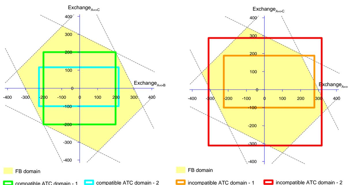
Figure 13 Compatible (figure in the left) and incompatible (figure in the right) FB/ATC domains
