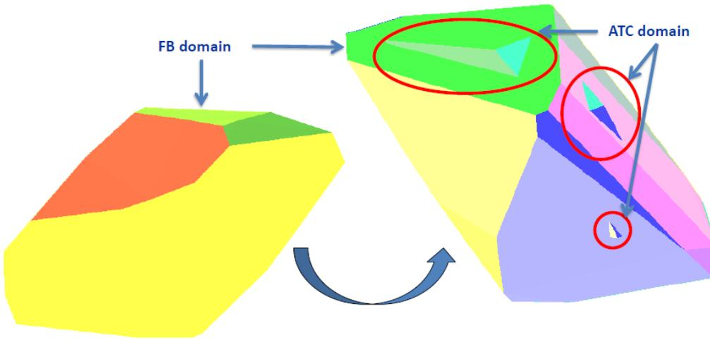
When a slice of these 3-dimensional bodies is made, the figure as shown hereunder could result (practical example of November 29, 10.30, 2010). The yellow polygon represents a slice of the ATC domain, whereas the slice of the FB domain is illustrated by means of its limiting critical branches.
