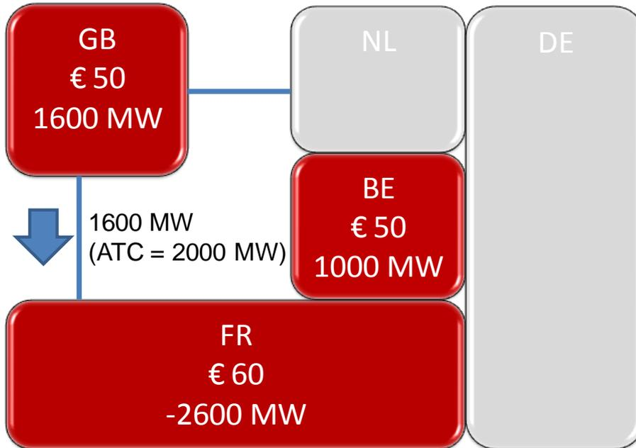
Figure 41: Example of advanced hybrid clearing with a price difference without ATC congestion.
